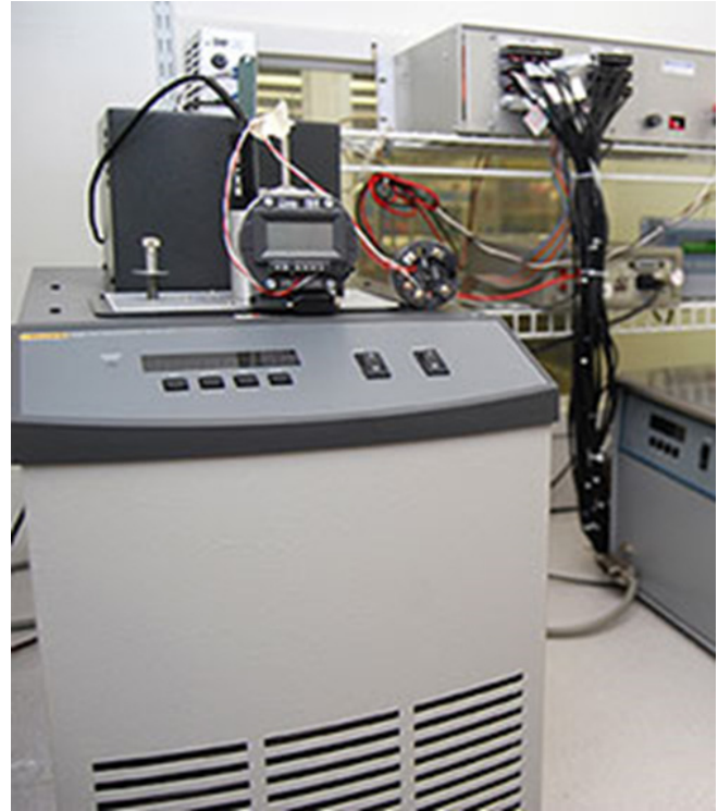
Figure 6. Temperature Transmitter Undergoes Bath Calibration
